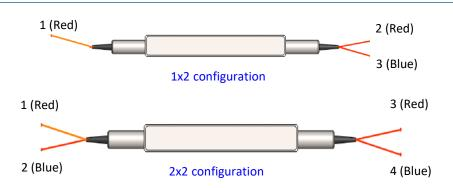
For 2x2 configuration, Port 1 -> port 3 and port 2 -> port 4 respectively without voltage. When a voltage is applied, the light from port 1 splits between port 3 and 4 and the light from port 2 splits between port 4 and 3, respectively with the same ratio. Portions of lights from port 1 and 2 incoherently add at output port 3 and 4 proportionally.
