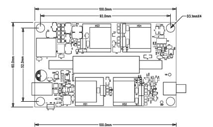
100kHz driver (100mmx60mmx11mm)
